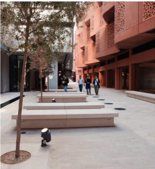
▼ Streets are narrow, for shade, and laid out to create cooling breezes. So it feels at least 15°C cooler here than outside the city.
