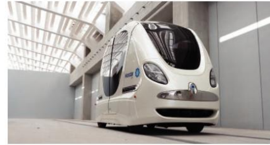
▲ Masdar City aims to be car-free at street level. They tried out these driverless electric pods for travelling under the city.
