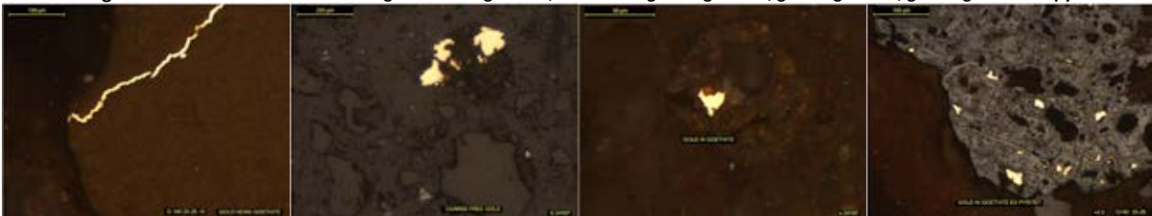
Figure 8: +2 mm slides – Hole G140 gold in aluminosilicates, gold in goethite, gold in goethite / manganese oxides, gold in kaolinsed schist
