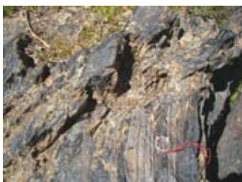
D – Hydrothermal breccia within a 075 trending structure cutting tourmaline altered sediments.
