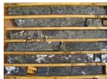
F – AD028 Tray53 (240.80m to 244.80m depth) shows the contact between the silica matrix supported hydrothermal breccia (upper part of tray to 243m) and the tourmaline altered sediment in matrix supported tectonic breccia (lower from 243m).
