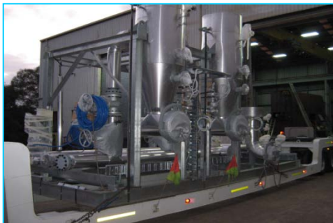
Panel 2 knock-out skid which forms part of the gas production facilities
