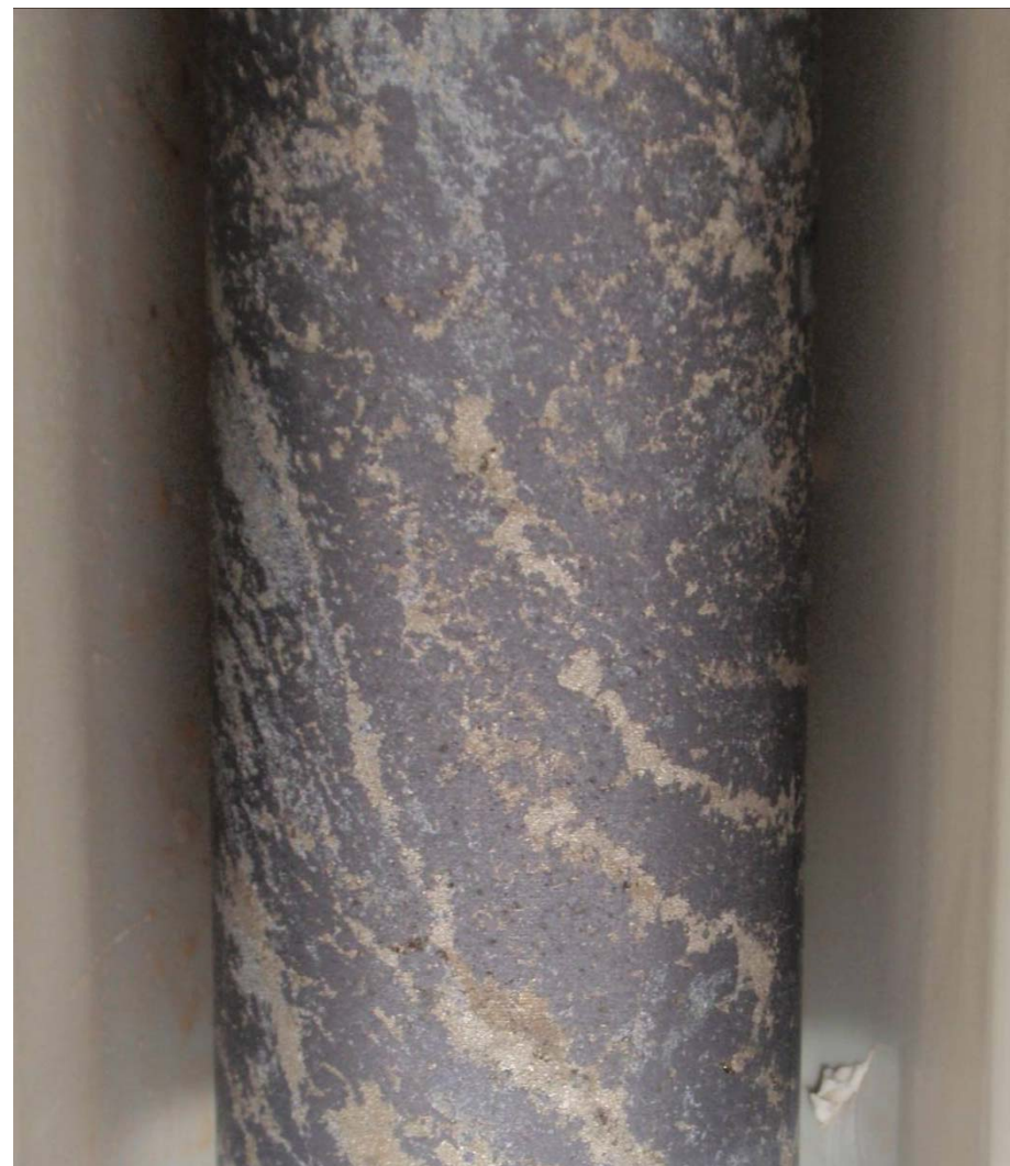
NEUDD001 - Intense magnetite alteration with pyrite stringers.
