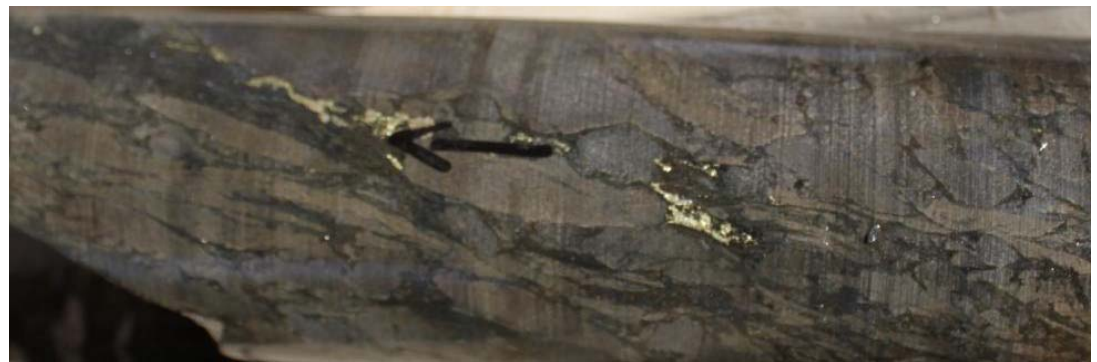
Chalcopyrite blebs and stringers within brecciated core from drill hole #AUGDD001 within the zone from 635m to 642m.
