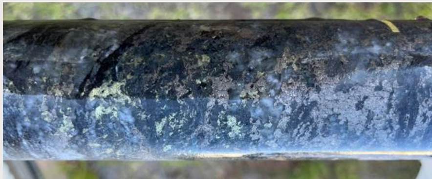
Chalcopyrite and pyrrhotite in BDCDD2501 at approximately 90m downhole
