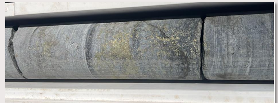
Chalcopyrite mineralisation in BDCDD2502 at approximately 237m downhole
