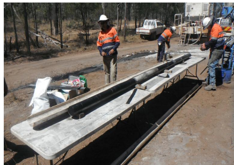
Coring by twinning open PCD hole ML0014 at Moorlands
