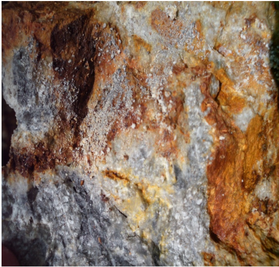
Figure 3: Silicified float (RF-009) shows quartz, pyrite and arsenopyrite.
