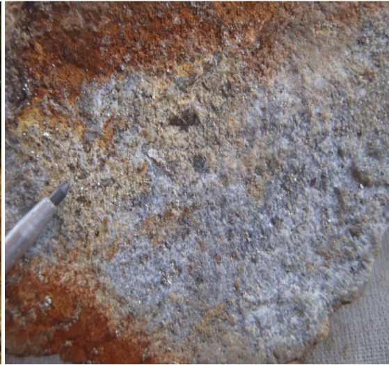
Figure 4: OC-010 silicified –argillic sandstone with disseminated pyrite and arsenopyrite.
