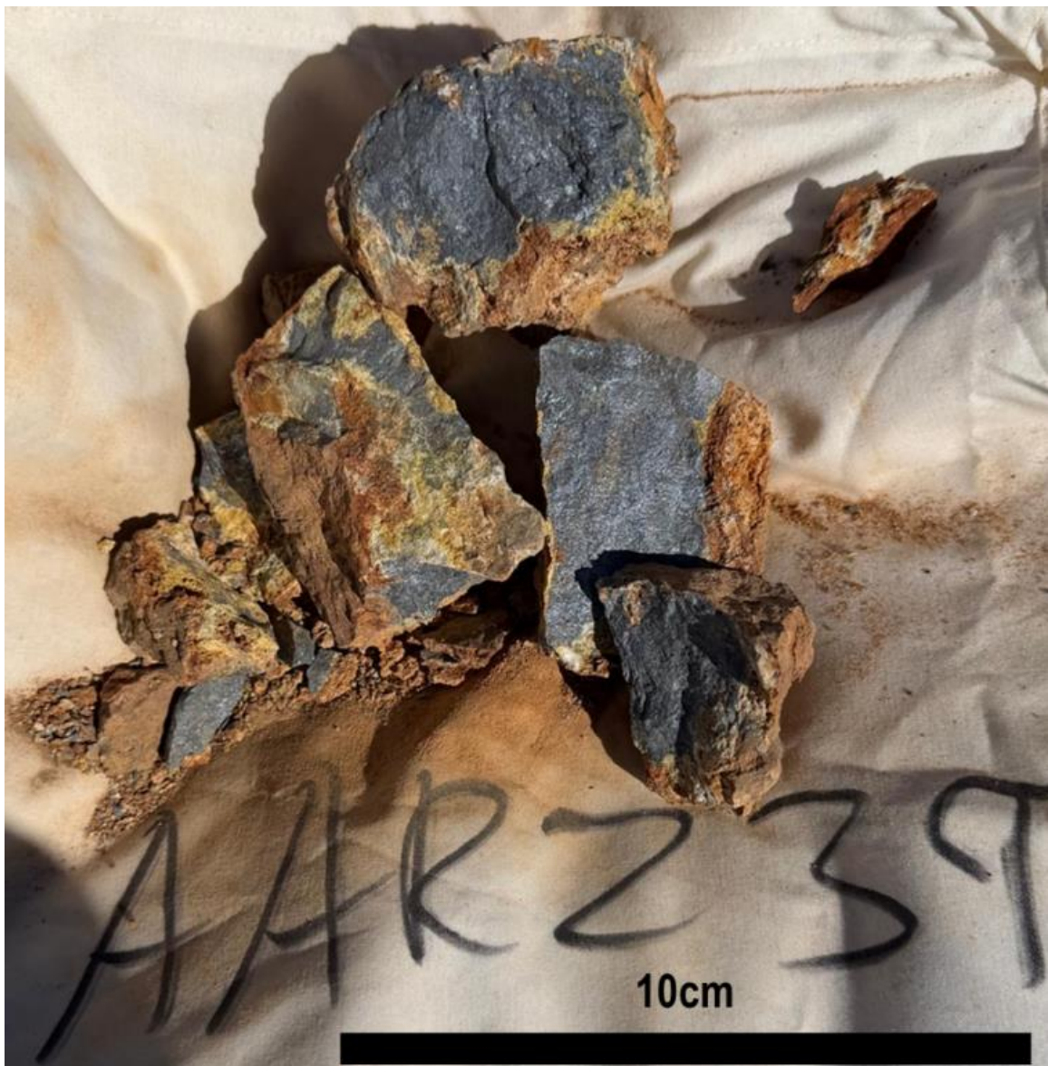
Figure 3: Sample of oxidised massive stibnite float (AAR239). The sample assayed 34.3% Sb. Refer to Table 1 for full analytical details.
