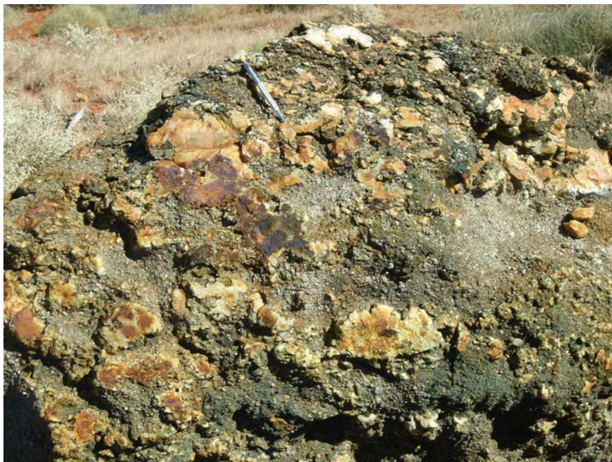
Fig.4 Breccia vein showing quartz clasts cemented by massive sulphide (pyrite and chalcocopyrite) from the Horseshoe pit
