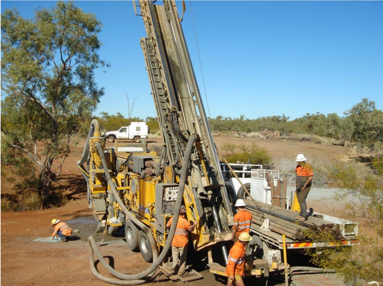
Fig. 2 RC drill rig operating in Duck Creek
