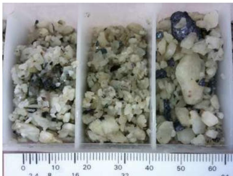
**Figure 2 – Molybdenite in NERC005 (68-70m) (blue/grey mineral)**
