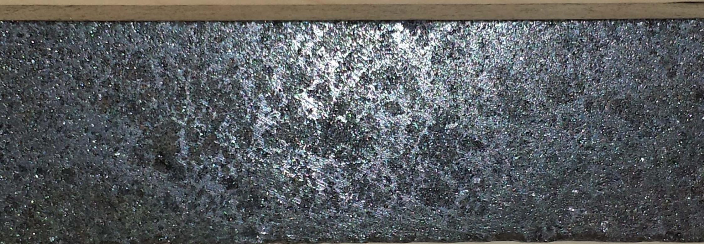
**Massive to semi-massive galena in carbonate and garnet schist**
