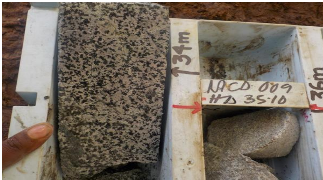
Figure 3. Typical photograph of the Wale Batholith (Tonalite) from 35.10m
