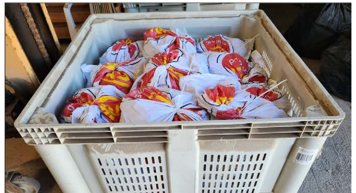
Figure 2: 690kg of sample ( 211kg oxide; 235kg mixed; 243kg sulphide) from the Pantanillo Gold Project ready for Metallurgical testing
