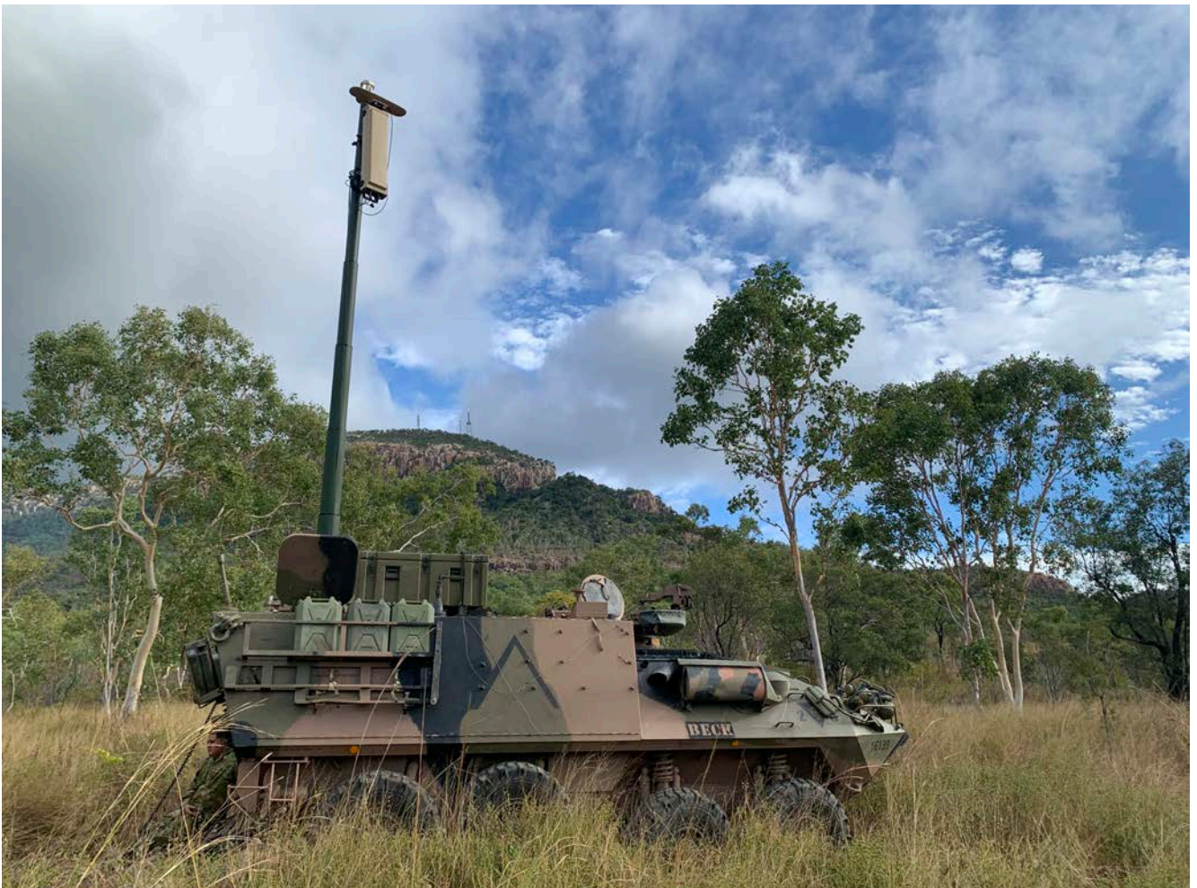
Image: DroneShield RfOne™ passive far-range drone detection sensors on an Australian Army vehicle
