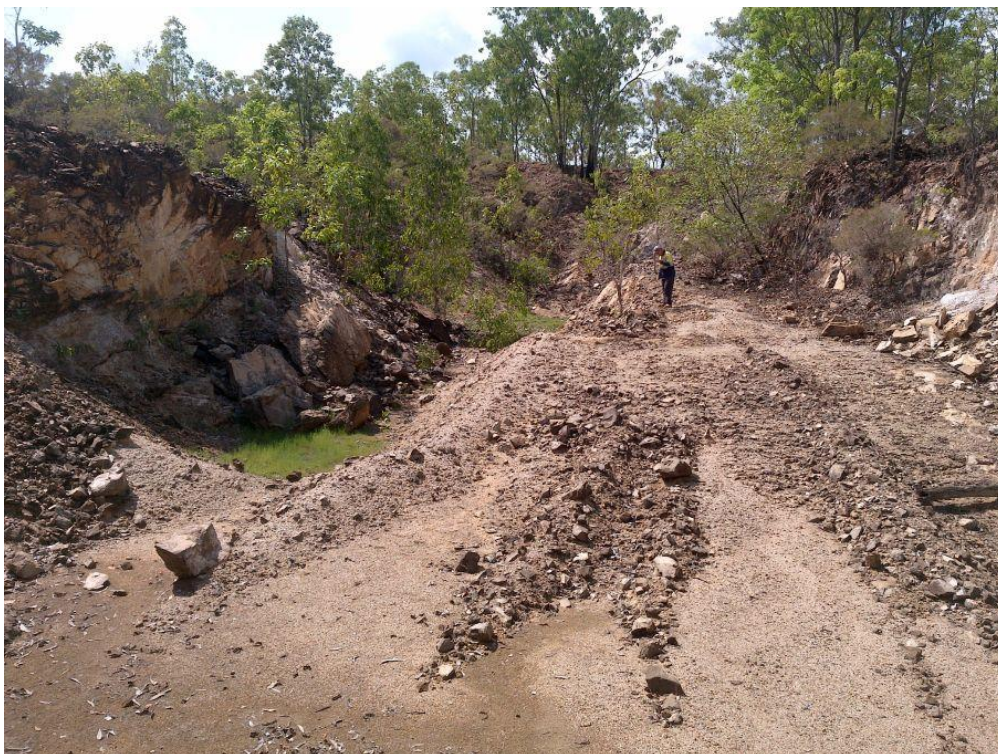
Figure B1. Booths Prospect open cut. Pegmatite dips at 40 degrees to the left of the frame (NE) and true width is approx. 20m at this location.
