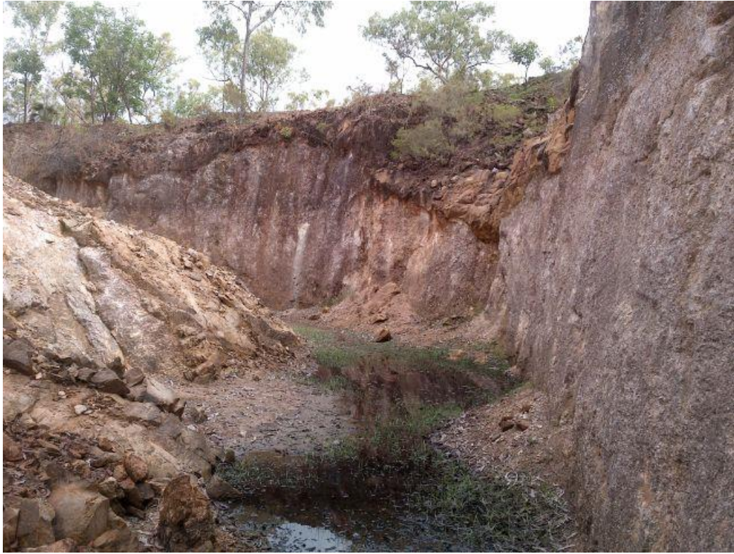
Figure LE3. Lees Extended Prospect open cut. Height of wall on right is approx. 25m. Pegmatite true width is approx. 12m
