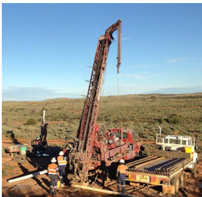
Diamond Drilling Pyrite Hill
