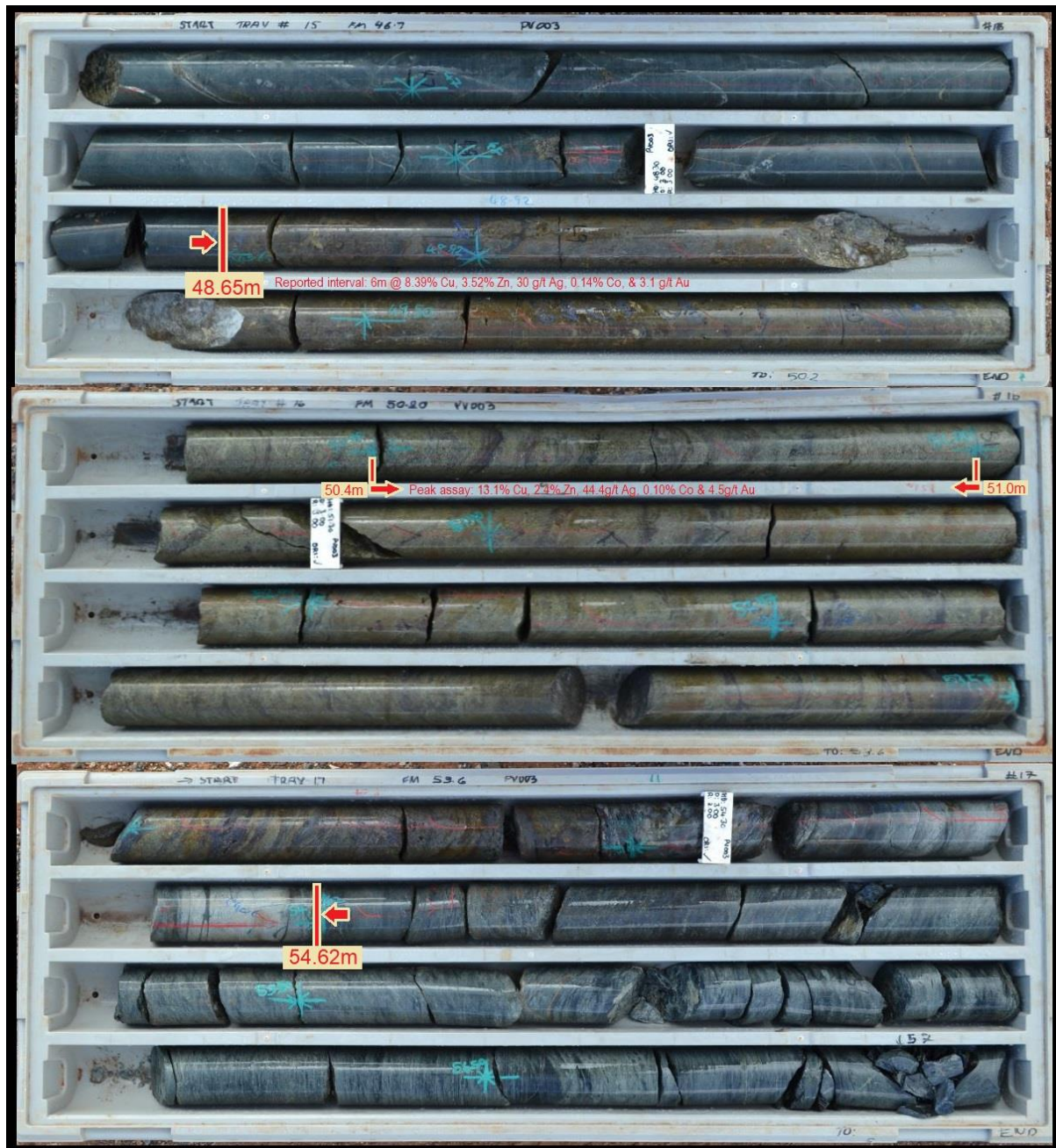
Figure 1: Core trays 15-17 from Schwabe drill hole 20PVDD003 containing primary VHMS from 48.65m to 54.62m
