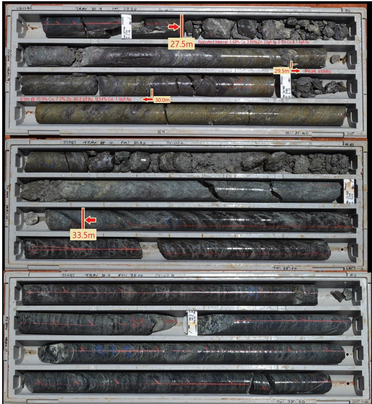
Figure 2: Core trays 9-11 from Schwabe drill hole 20PVDD004 containing VHMS from 27.5m to 33.5m (note: core run from 27.4m to 30.4m includes 30% core loss)
