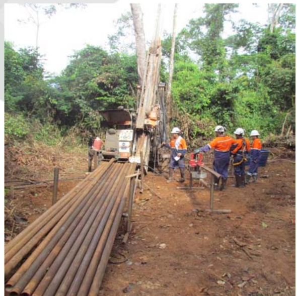
Figures 1 and 2: Drill rigs arriving on site and collaring the first hole at Querosene
