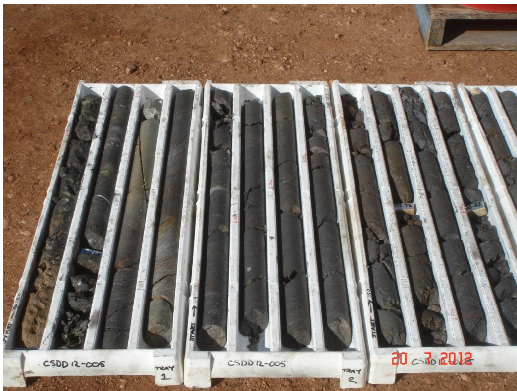
Plate 3. HQ drill core of highly graphitic schist in hole CSDD12_005
