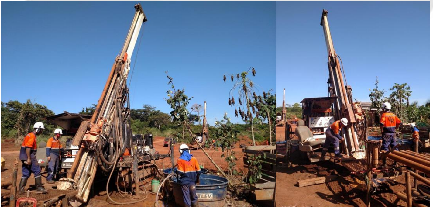
Figure 2: Images of ongoing diamond drilling campaign at Juruena project, Brazil.
