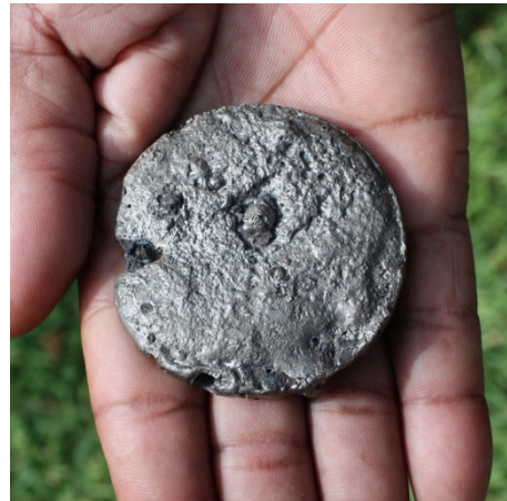
Plate 1: Disc of Baobab pig iron
