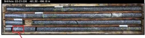
GD-23-226 - 431.50 - 496.10 m (2024 - Resampling) - Coarse grained porphyritic intermediate intrusive with thin quartz veinlets with calc-silicate haloes. Veins include minor native bismuth, molybdenite, pyrrhotite, pyrite, and native gold, all no more than 1%.
