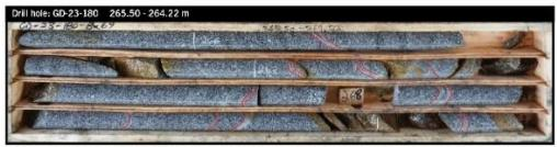
GD-23-180 - 265.50 - 264.22 m (2024 - Resampling) - Quartz veins with calc-silicate haloes, up to 4 veins per meter. These veinlets and haloes have a rare amount of pyrrhotite and rare sphalerite.
