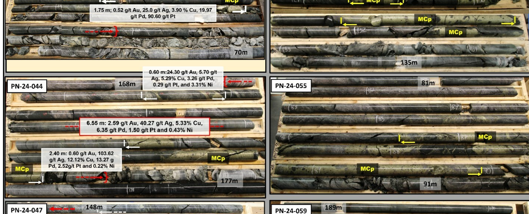
Figure 2: Core picture of hole PN-24-047 showing the strongly mineralized intervals and its location on a vertical cross-section view looking ENE along holes PN-24-047 and PN-24-051.
