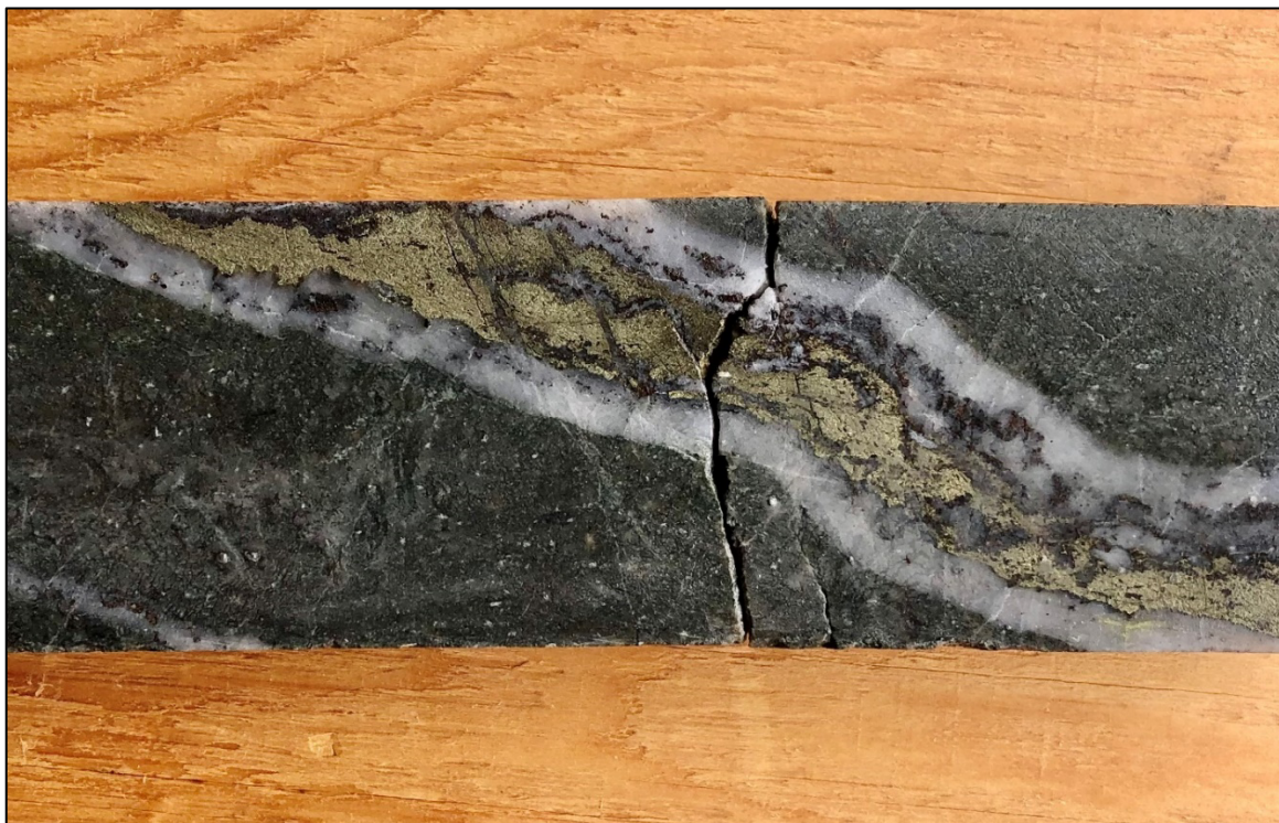
Figure 4: Example of core from 2022 drilling at Gate Zone, hole MPD-22-006 . Quartz vein with centerline of chalcopyrite and bornite in hornblende-phyric diorite host rock at 696 metres. Core is within a 117 metre intercept reporting 0.69% Cu, 0.46 g/t Au and 2.22 g/t Ag from 587 to 704 metres
