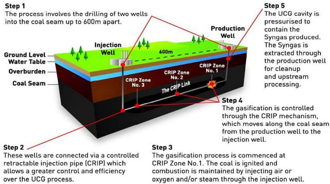
Clean Global Energy's advanced Linear CRIP (Controlled Retractable Injection Point) UCG process provides greater efficiencies and control with less overall operating and capital costs.
