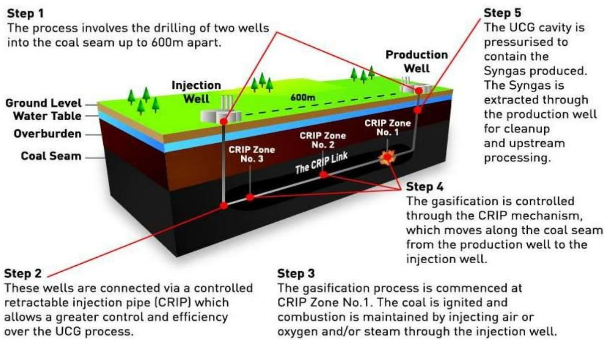
Clean Global Energy's advanced Linear CRIP (Controlled Retractable Injection Point) UCG process provides greater efficiencies and control with less overall operating and capital costs.
