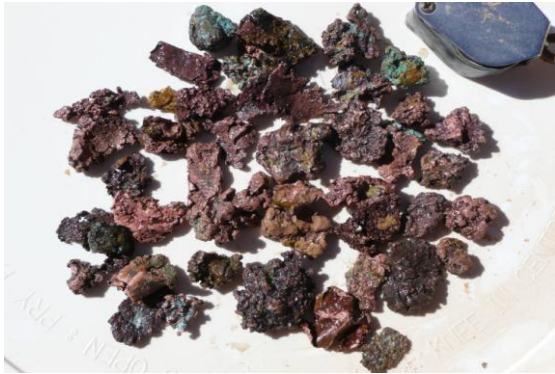
Nuggets of native copper derived from processing of Kalkaroo drill chip samples in the test plant
