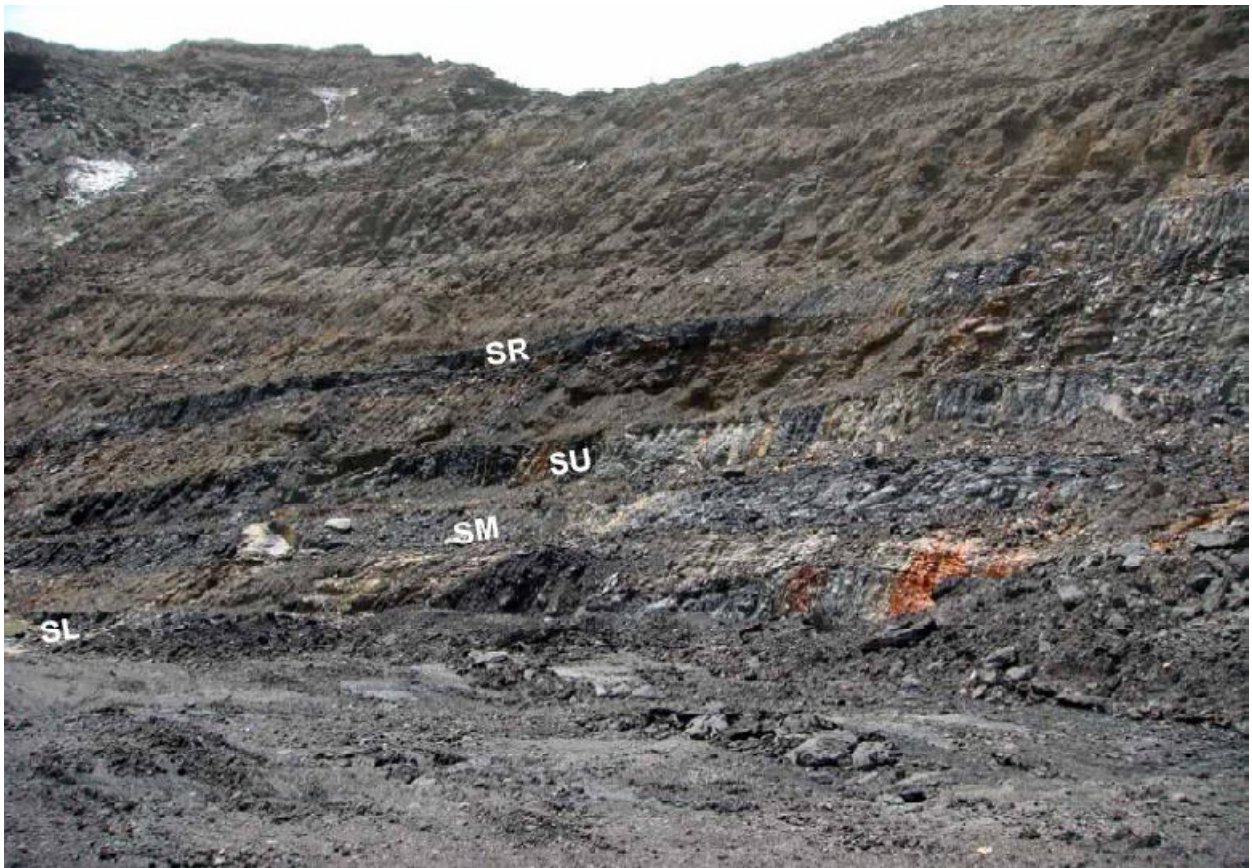
Figure 9 – Four exposed coal seams dipping into the TCM area.
