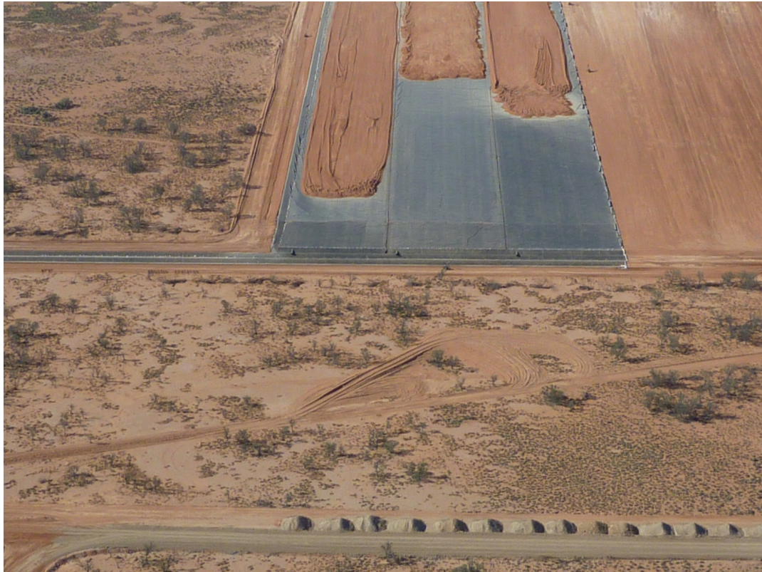
Figure 4: WDGPJV earthworks for leach pads
