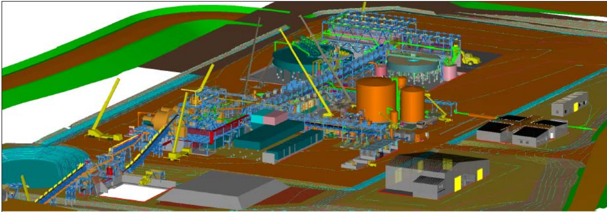
Figure 1: Concentrator model viewed from crusher end showing construction cranes
