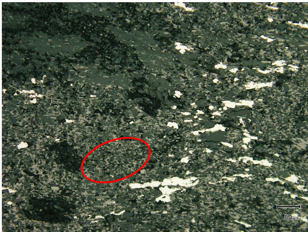
Plate 5. SLRC11_001 128 to 129m, very fine graphite flakes circled. Brightest material is sulphide.
