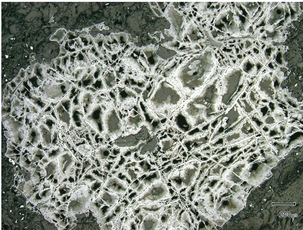
Figure 1. Polished section (PS), (x50). Gossanous/goethite box-work with a fine trellis texture interpreted to represent original chalcopryite now completely oxidised and leached.
