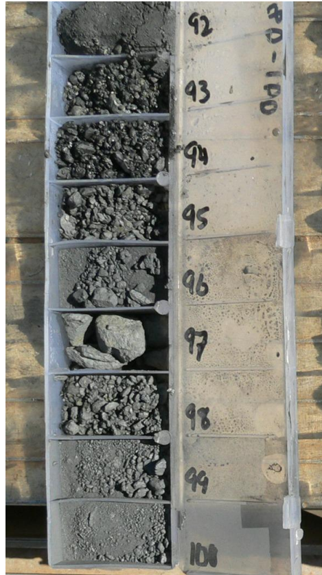
Figure 6 Graphitic intervals from SLRC11_004, note, the rocky nature (93-96m) is due to the sample being sieved and washed, before being placed in the chip tray, intervals 92 and 100 are representative of what is recovered from drilling.
