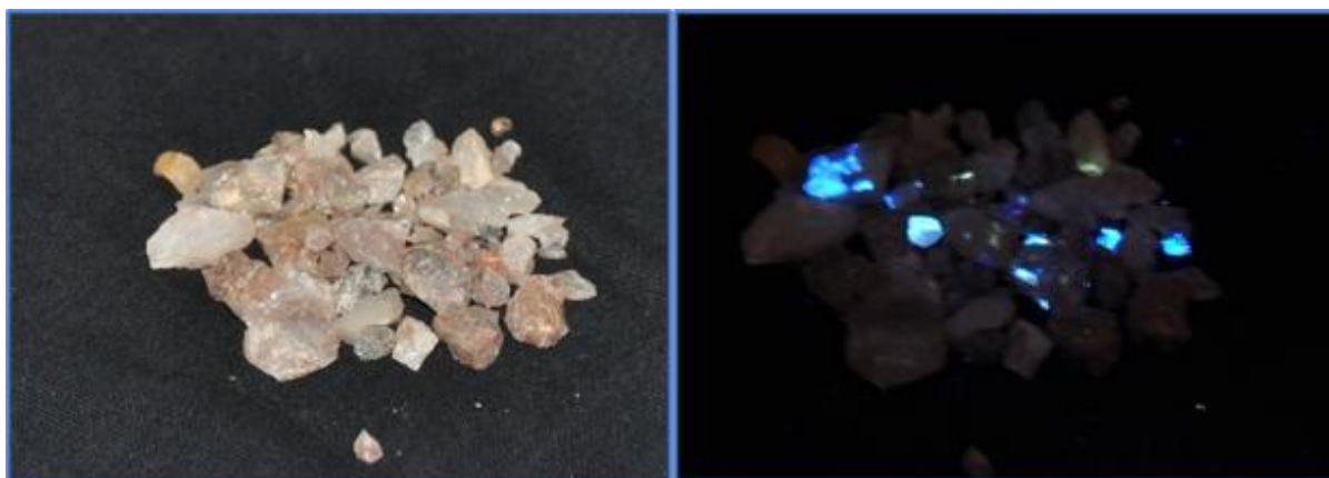
Figure 1: Sample MPL21_559 under natural (left) and UV (right) light highlighting scheelite (tungsten) luminescence, with individual scheelite grains up to 8 mm in size
